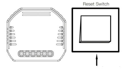
Note:This smart switch module can only be used with reset switch.
