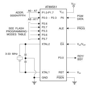
Figure 17-1. Programming the Flash Memory (Parallel Mode)
