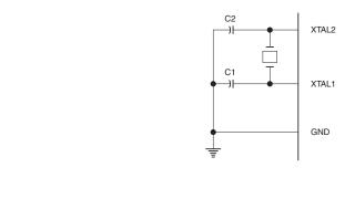
Note: C1, C2 =  $30 \text{ pF} \pm 10 \text{ pF}$  for Crystals =  $40 \text{ pF} \pm 10 \text{ pF}$  for Ceramic Resonators
