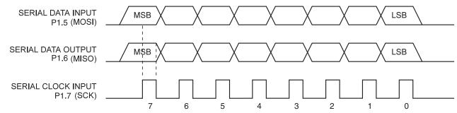
Figure 19-1. Serial Programming Waveforms
