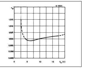
Figure 11. Propagation delay versus voltage level of trigger value
