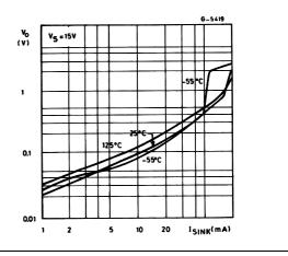
Figure 9. High output voltage drop versus output
