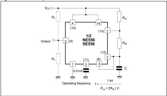
$t_1 = 0.693 (R_A + R_B) C$  output high
