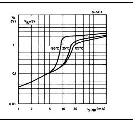
Figure 7. Low output voltage versus output sink current
