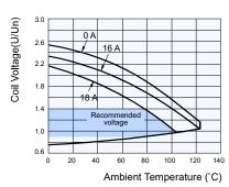
Notes: \* The use of a relay with an energising voltage other than the rated coil voltage may lead to reduced electrical life.
